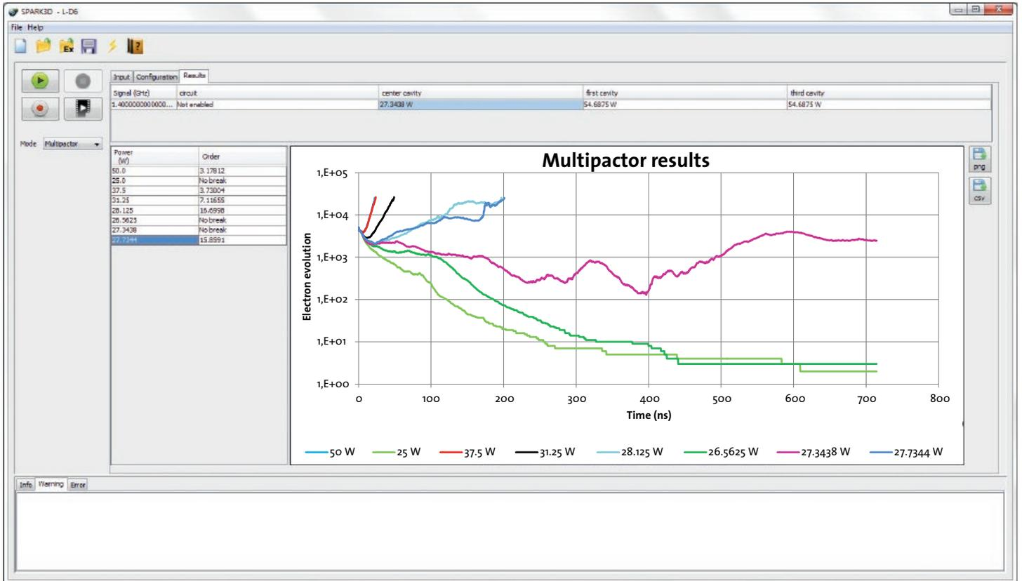
Figure 5: SPARK3D interface showing the multipactor breakdown results for this particular component with electron evolution over time for different power levels.
