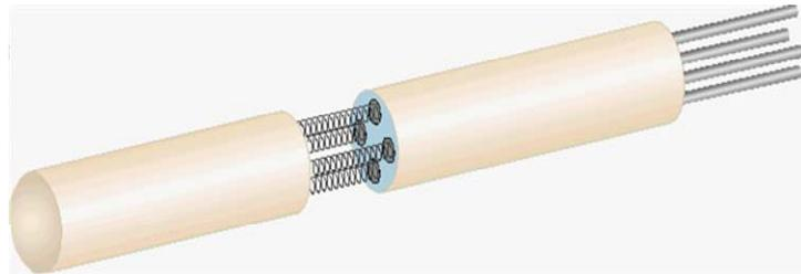
The most common RTD element material is Platinum, as it is a more accurate, reliable, chemically resistant, and stable material, making it less susceptible to environmental contamination and corrosion than the other metals. It's also easy to manufacture and widely standardized with readily available platinum wire available in very pure form with excellent reproducibility of its electrical characteristics. Platinum also has a higher melting point, giving it a wider operating temperature range.
