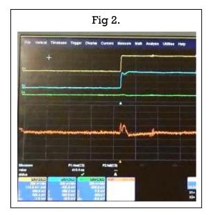
Starting with **Figure 2** you can see the demonstration of the problem and the output pulse shape initial conditions. The yellow pulse is the input RF pulse, the amplifier output and its nonlinear response is in Blue. The Orange trace is the error between the Yellow and Blue signal, including the rising edge slope (not to scale). The Green trace is the accumulated applied inverse error.
