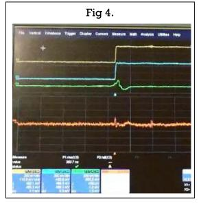
Again, on the next cycle, **Figure 4** shows the remaining error applied. The output pulse virtually matches the input. The accumulated applied error is larger (Green) and the present state error is smaller (Orange). The loop runs continually while adjusting for any present conditions in the error function, including droop.
