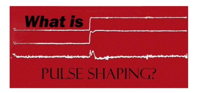
By George Bollendorf Empower RF Systems Pulse shaping, as it is done today, is an effort to fix fidelity issues caused by the transmitting amplifier and is accomplished by a combination of imperfect methods, most external to the amplifier. In this industry briefing George Bollendorf explains a new approach that matches input pulse signal shape, minimizes droop, overshoot, ringing, rise and fall times.
