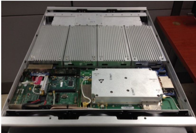
Air Cooled RF Deck
