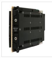
The 5586 is a high-performance, SOSA aligned 3U OpenVPX coprocessor board based on the Xilinx Virtex UltraScale+ HBM FPGA. It serves as an ideal stand-alone processor or as a co-processor for distributed FPGA processing tasks.
